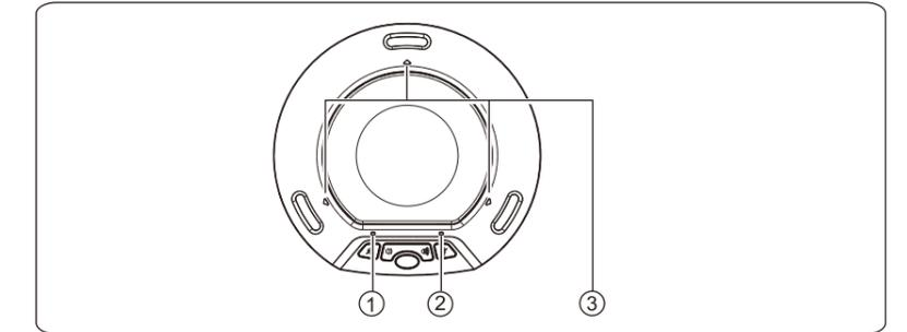
**1. Bottom left indicator:** When the loudspeaker gives out sound normally, the light is off; when the loudspeaker is muted, the light is on; when the loudspeaker is adjusted to the maximum/minimum volume, the light will blink.
