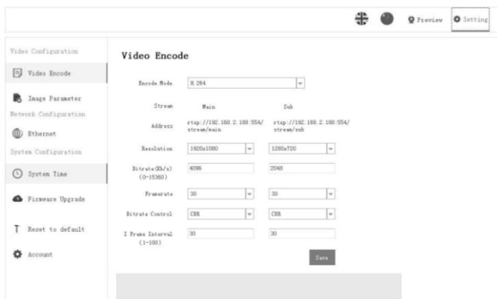
“Video Encode ”: can set image encode mode, main stream and sub stream resolution/bit rate/frame rate, bit rate control way, and I frame interval etc as above image
