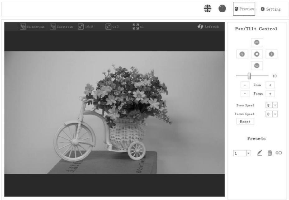
Preview interface as above image, on the right side, there are options to control camera pan, tilt, zoom, focus, presets, focus speed, zoom speed can be set. On the top of the image, main stream and sub stream preview can be selected, image width&height rate can be selected, and full size view can be selected. Besides, English and Chinese language is optional.
