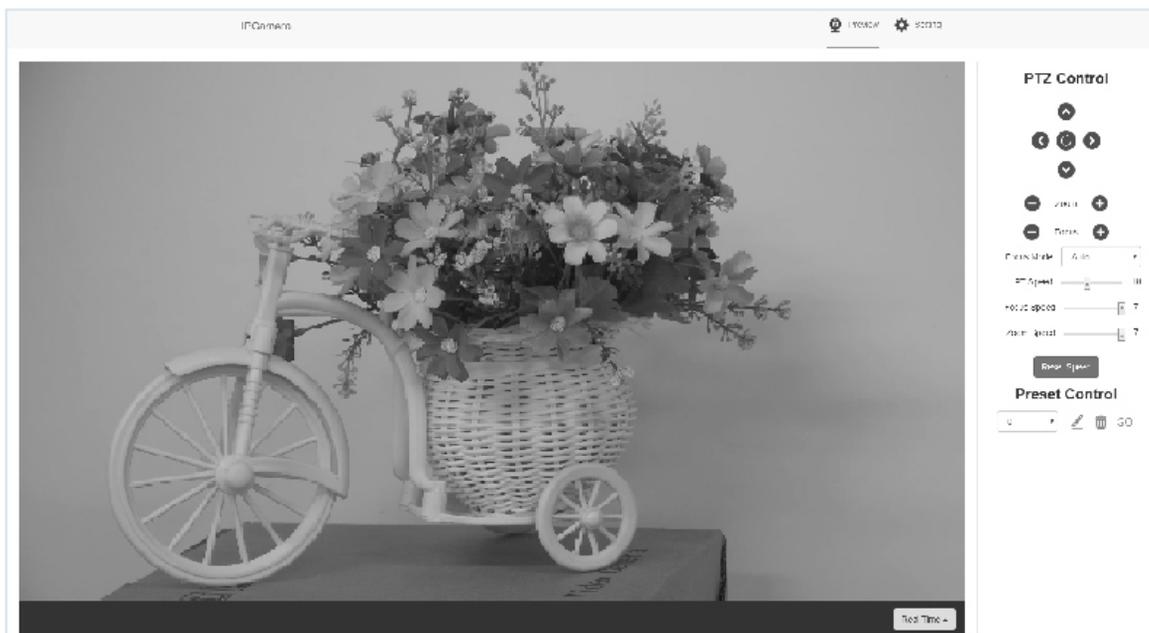
Preview interface as above image, on the right side, there are options to control camera pan, tilt, zoom, focus, presets, focus speed, zoom speed can be set. On the top of the image, main stream and sub stream preview can be selected, image width&height rate can be selected, and full size view can be selected.
