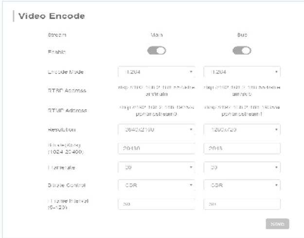
“Video Encode”: can set image encode mode, main stream and sub stream resolution/bit rate/frame rate, bit rate control way, and I frame interval etc as above image
