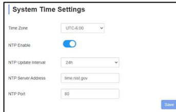
The screenshot shows a form titled "System Time Settings". It contains several settings: "Time Zone" set to "UTC-6:00", "NTP Enable" checked, "NTP Update Interval" set to "24h", "NTP Server Address" set to "time.nist.gov", and "NTP Port" set to "80". A blue "Save" button is located at the bottom right of the form.
