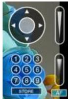
Refer to above picture, once open the video via Studio Monitor, it will show up the control panel on the right side, to control camera pan, tilt, zoom, focus, preset, focus.
