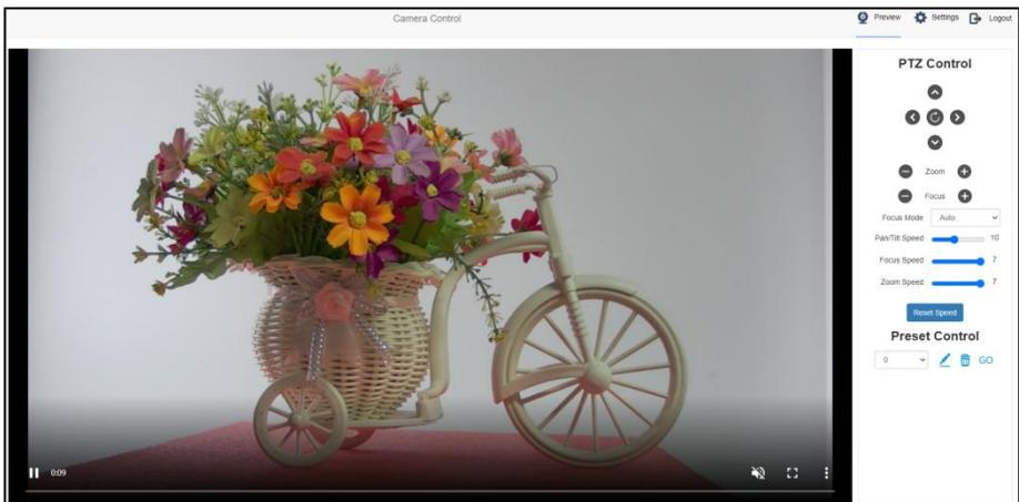
The preview interface is shown above. On the right side, there are options to control camera pan, tilt, zoom, focus, focus mode, pan tilt speed, focus speed, zoom speed, preset position control, etc. At the bottom of the image, you can
